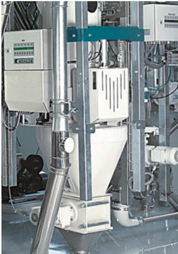
Automatic MSDL hopper scale with MEAG universal control unit.
