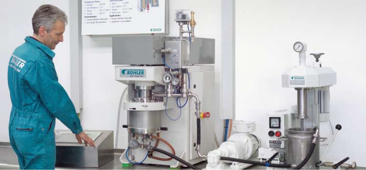
Fig. 8.1: SuperFlow® 12 pilot Perl Mill® with control package PREMIUM and complete setup for recirculation operation
