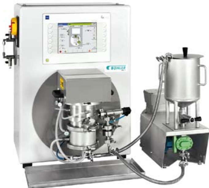
Fig. 11.3: SuperFlow® 4 in recirculation operation
