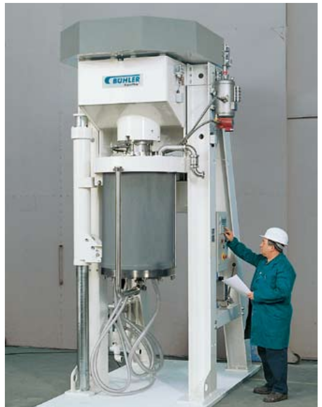
Fig. 5.3: SuperFlow® 800 – Large-volume Perl Mill® for the nano-grinding of pigments, 250 kW drive with grinding chamber volume of 79 l
