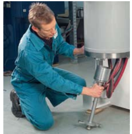
Fig. 9.3: Removal of protective screen from a SuperFlow® VCR 200 filled with grinding media
