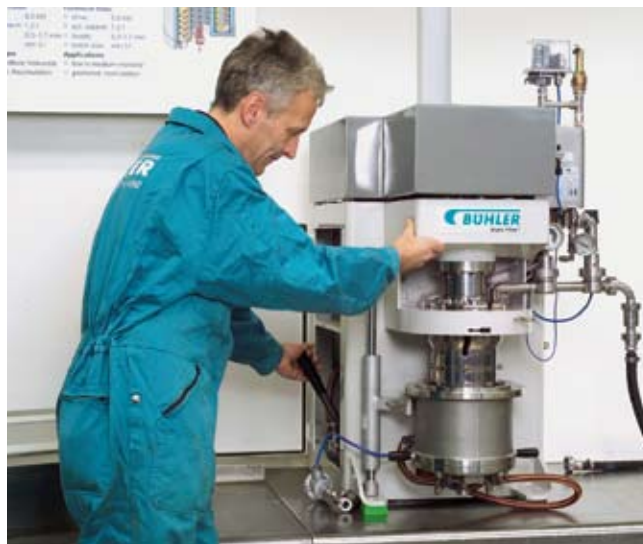
Fig. 4.2: SuperFlow® 12 while lowering of grinding vessel
