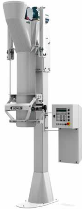
Automatic auger packer – for compacting non-freeflowing, bulky products.
