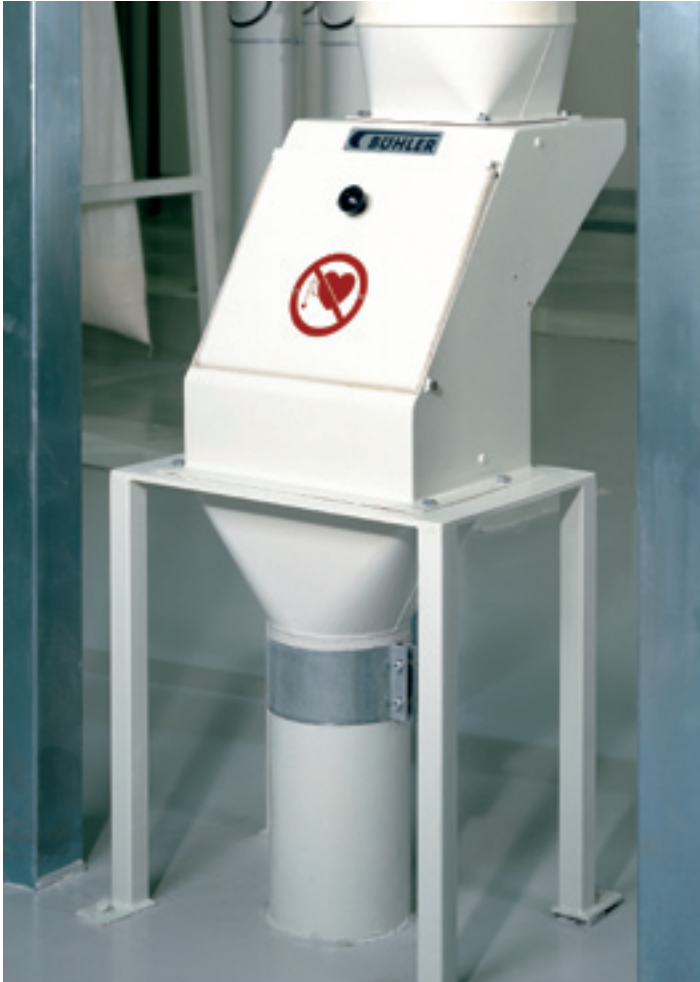
Magnetic Separator MMUA. For the removal of iron parts.
