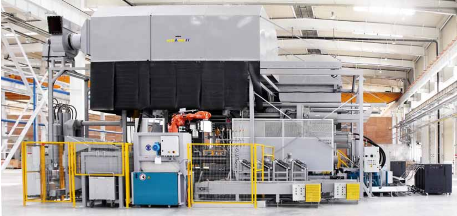
One of the two new die casting cells of GWM.
