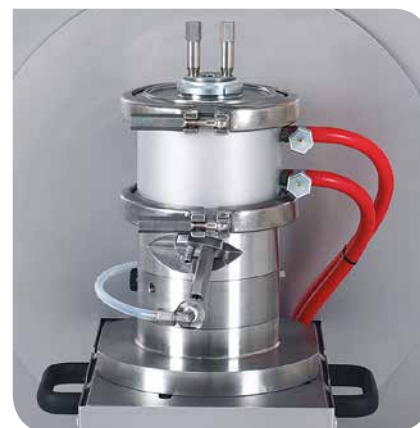
Service position for mounting of the process unit, filling of the grinding beads and cleaning
