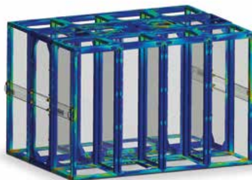
FEM calculations for the Arenit sifter frames.
