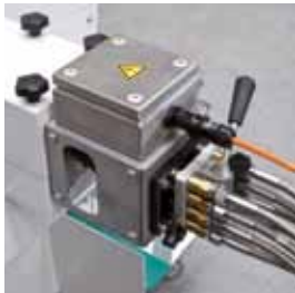
Multiple coupling for fast drum maintenance and cleaning.
