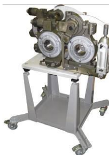
Wagon for bearing unit change only for MDDR / MDDT / MDDM / MDDO
