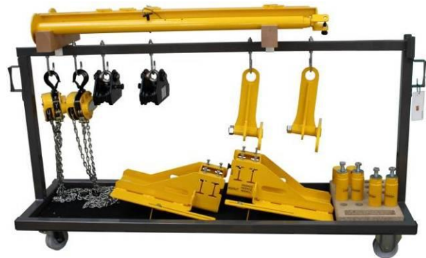
Transport carriage with all parts of the Universal Lifting Device
