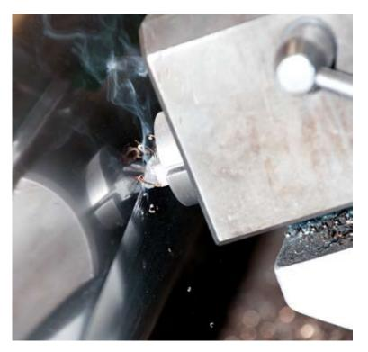
The corrugating machine cuts highly accurate corrugations into the rolls. The differences in the number, geometry, twist, and position of the corrugations produce over 10,000 variants – carefully matched to the specific production process.
