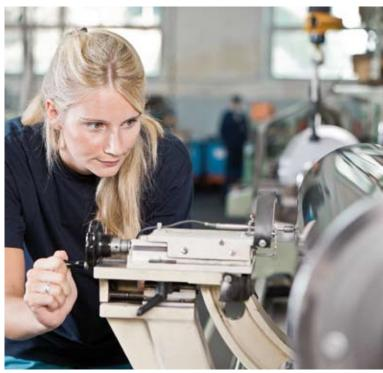
Buhler cambers the rolls as required by customers. In the subsequent camber test, the rolls are checked to one thousandth of a millimeter.
