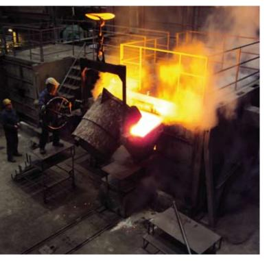
Narrow process parameters ensure a consistently high quality as early as in the casting process – as here during tapping of the molten steel.
