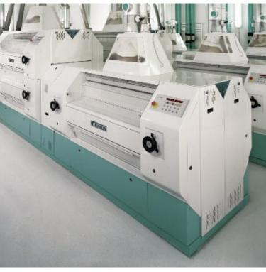
**Buhler grinding technology** covers a wide range of requirements. Roller mill grinding for well controlled size reduction or impact grinding for high capacities and a high portion of fines.
