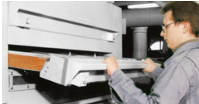
The different sieves are easy to exchange, despite their sturdy design.
