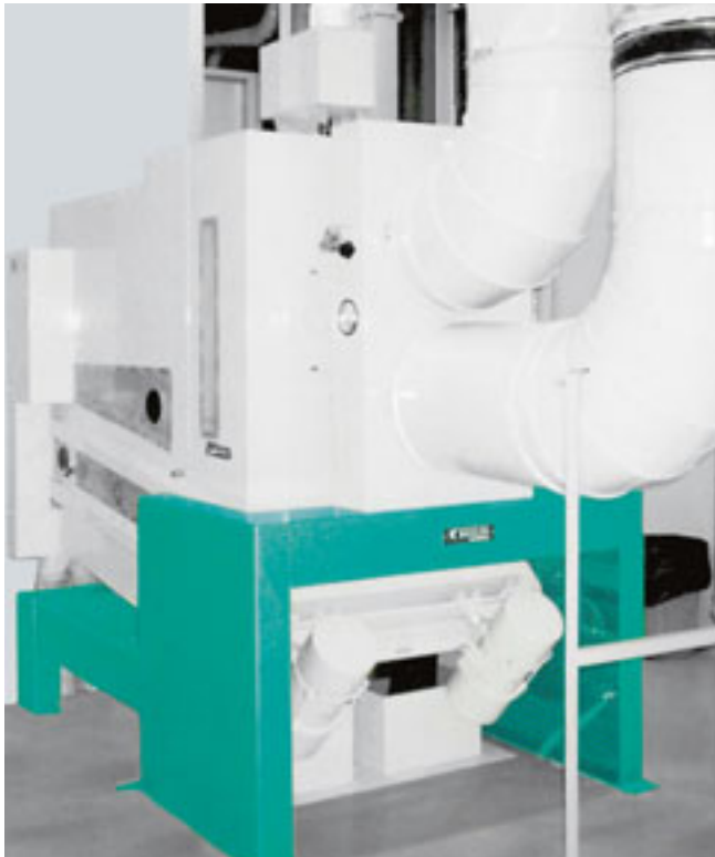
The entire sieve support is driven by two synchronized vibrators.
