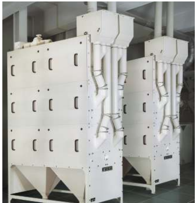
Line of two Rotosort™ in a large capacity rice mill - a modular DRGA-3D configuration
