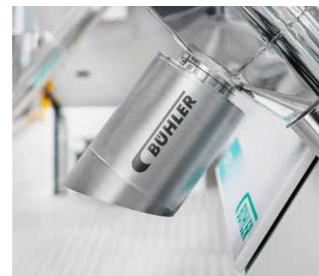
Installation of the measurement probe on a gravity spout.
