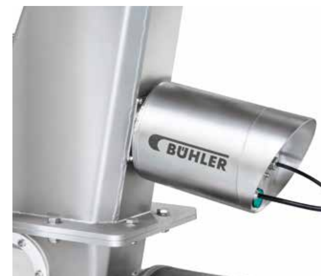
Installation of the measurement probe on a retarding section.
