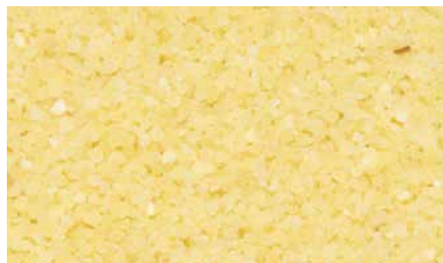
Color checking during ongoing production (L* 85,46 / a* -0,73 / b* 36,52).
