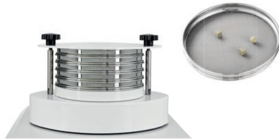
Standard sieve set for brewery applications according to MEBAK and EBC
