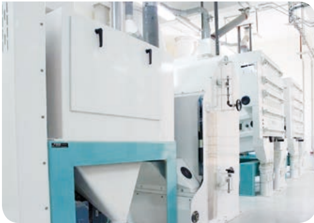
Excellent scouring effect. Scourer MHXS with air-recycling aspirator MVSQ.
