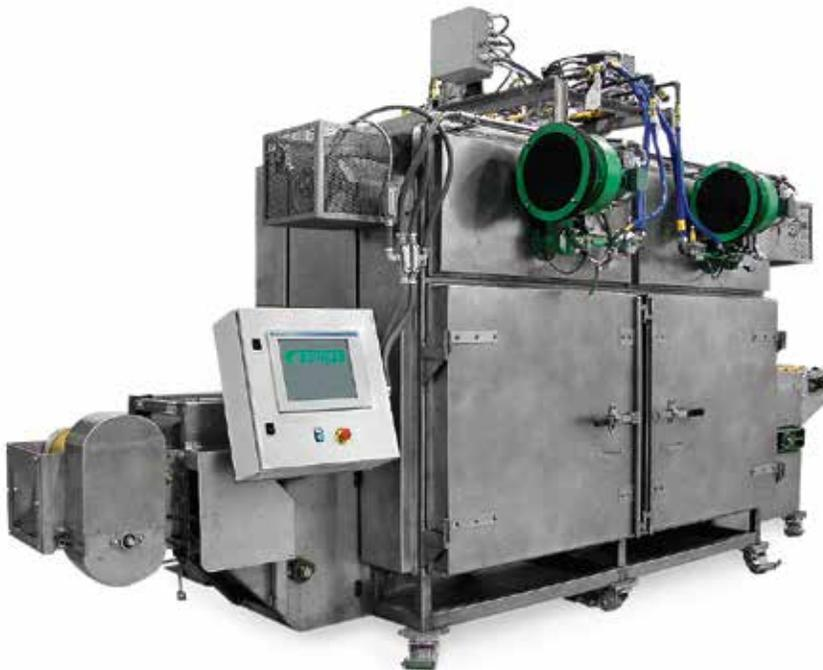
The continuous lab dryer is capable of pilot scale product testing in several configurations including dual impingement, through-air and fluidized bed. In addition to testing at the Bühler Aeroglide lab, customers may lease the lab dryer or other equipment for use at their facility.
