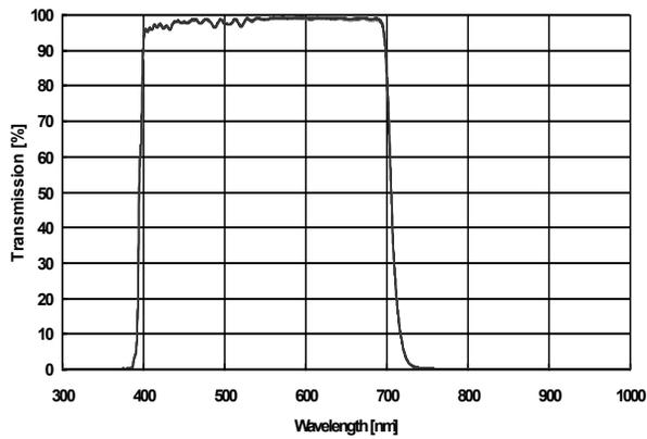
**Fig. 3** Performance of a dichroic UV-IR cut filter deposited with the HELIOS sputter system. The design consist of 52 non quarter wave layers, all layers are time controlled
