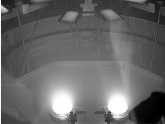
**Fig. 1** Tandem plasma source solution: Two Advanced Plasma Sources running in a SYRUSpro
