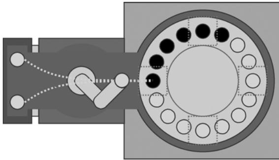
**Fig. 2** HELIOS sputtering system: Substrate handling and turntable
