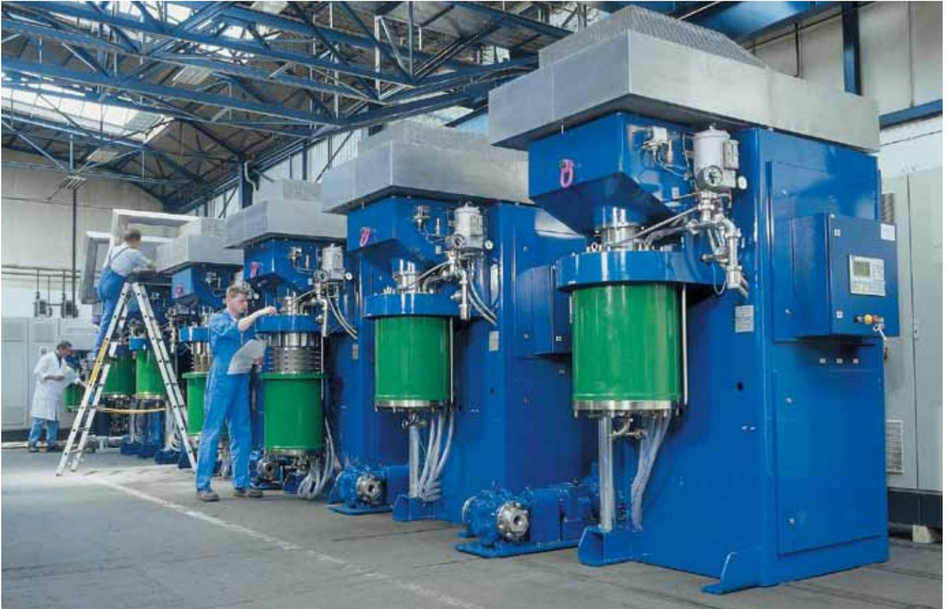
Fig. 5.1: SuperFlow™ VCR 400 with special painting: High-performance recirculation bead mill for the manufacture of concentrates.
