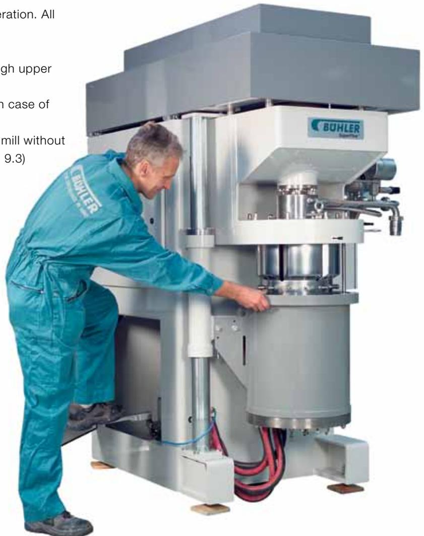
Fig. 9.4: Foot-operated hydraulics for lifting of grinding vessel of a SuperFlow™ VCR 200.
