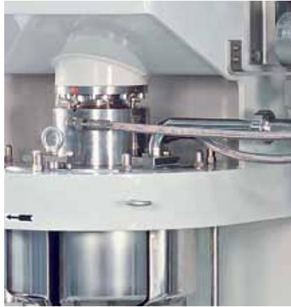
Fig. 9.2: SuperFlow™ VCR 200 – grinding vessel lowered and pivoted.
