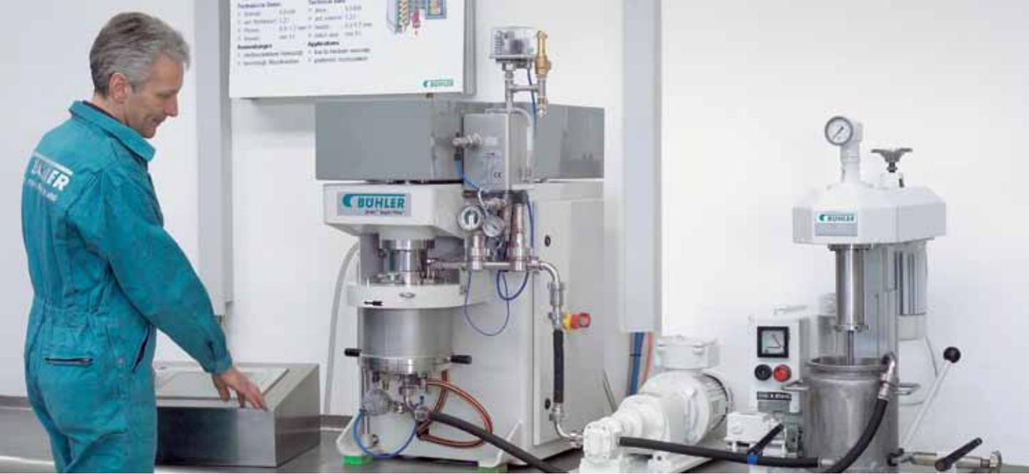
Fig. 8.1: SuperFlow™ 12 pilot bead mill with control package PREMIUM and complete setup for recirculation operation.
