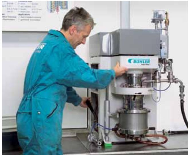
Fig. 4.2: SuperFlow™ 12 while lowering of grinding vessel.
