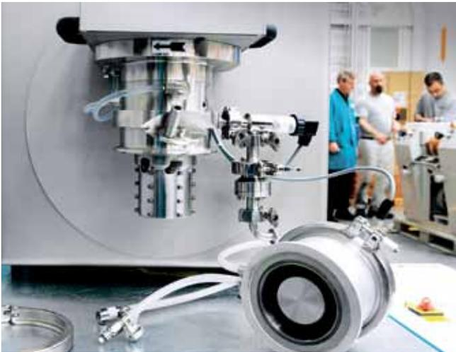
Fig. 11.1: SuperFlow™ 4 with removed grinding vessel.
