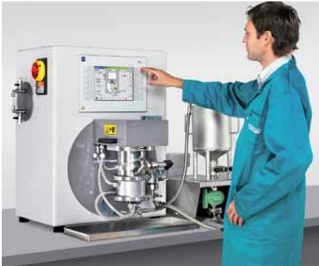
Fig. 4.1: Lab mill SuperFlow™ 4 with control package PREMIUM and complete setup for recirculation operation.
