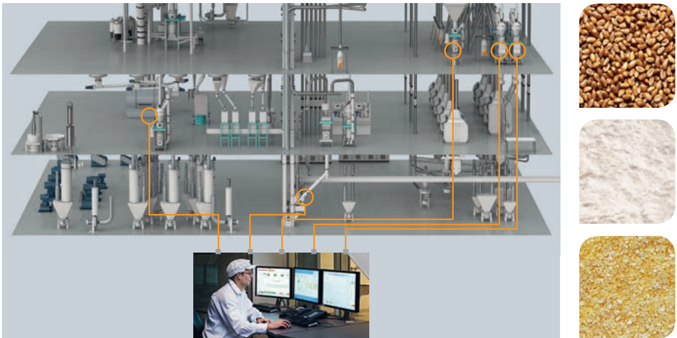
Online measurement of whole grain, flour, and semolina.
