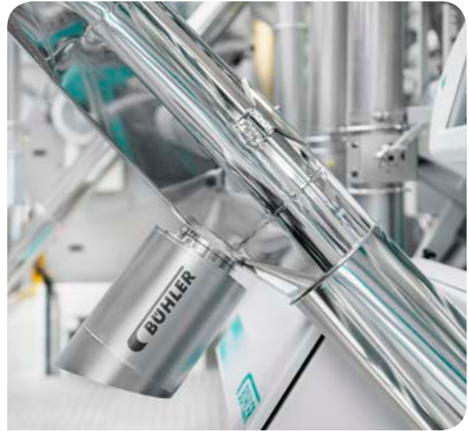
The color and speck measurement option MYHB delivers reproducible color values in the CIE 1976 color space (L*, a*, b*) and classifies brown as well as black specks according to size.
