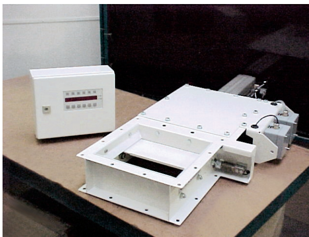
Feed gate without inlet and outlet components MEAF control system can be installed remotely from the slide gate (max. 10 m cable length).
