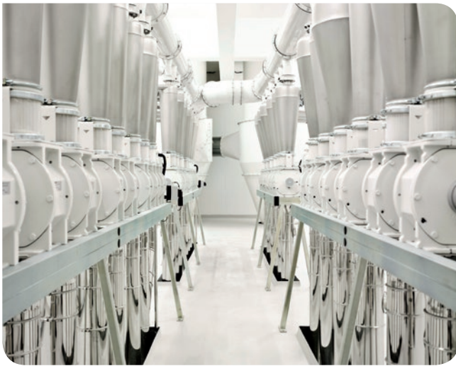
Pneumatic mill stock: airlock table with cyclone and discharge airlock MPSN.
