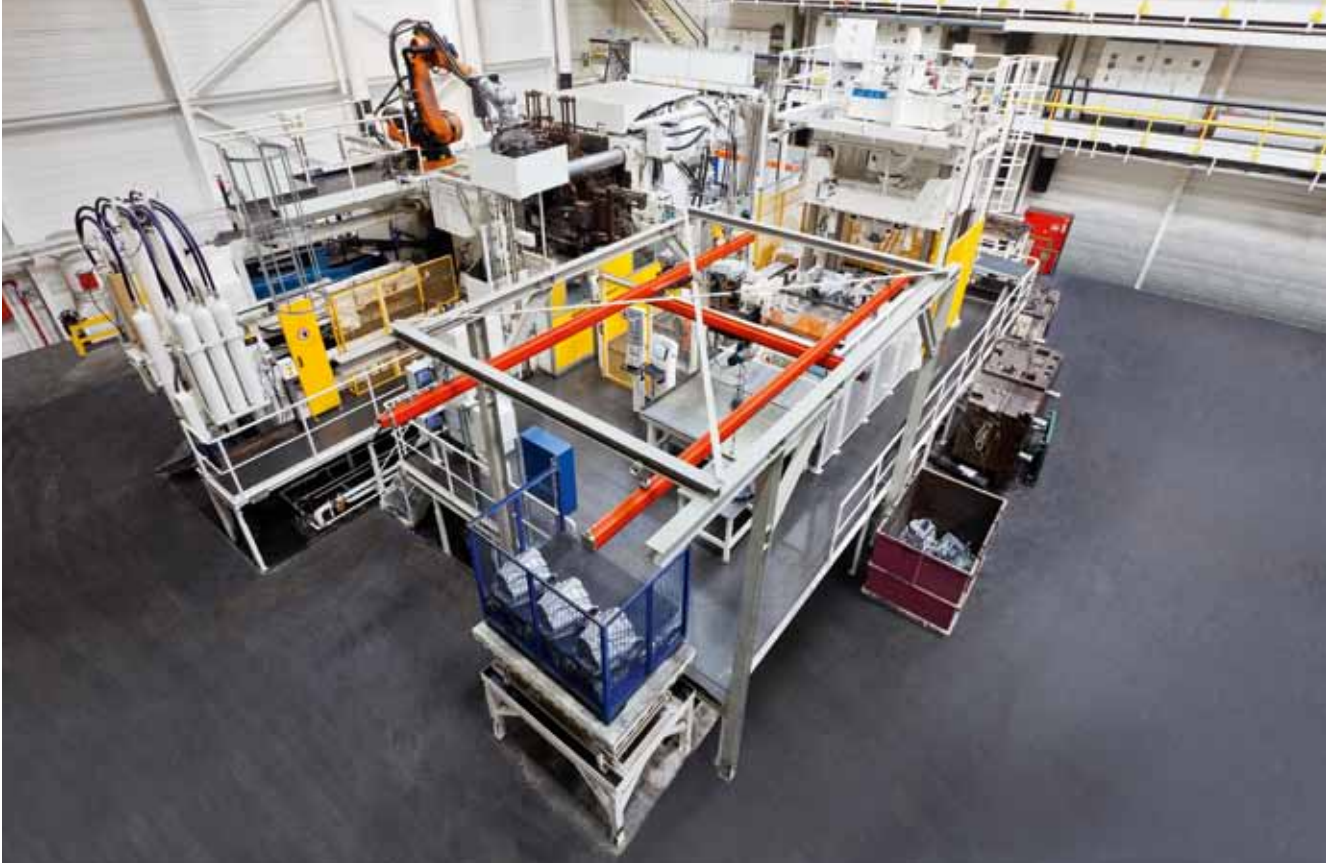
The two-platen die casting system of type Carat 440 in the Volkswagen factory in Kassel.
