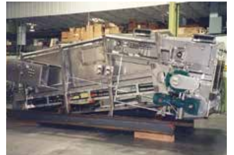
Apron feeder converts multiple batches into continuous flow
