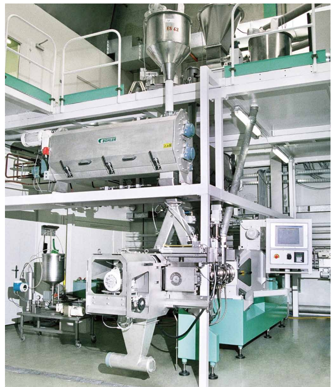
The Buhler extruder used in the NutriRice process. Photos courtesy of Buhler.
