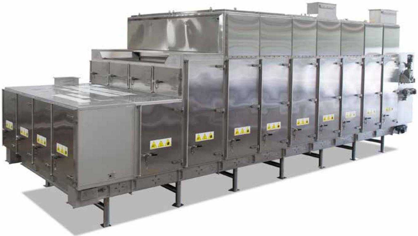
Bühler's Solis conveyor dryer has a unique dual plenum airflow that distributes heat and air uniformly to both sides of the product bed. This maximizes heat transfer to keep operating efficiency high and utility costs low. Independently controlled heating zones maximize processing flexibility and ensure the exact product specifications are met.
