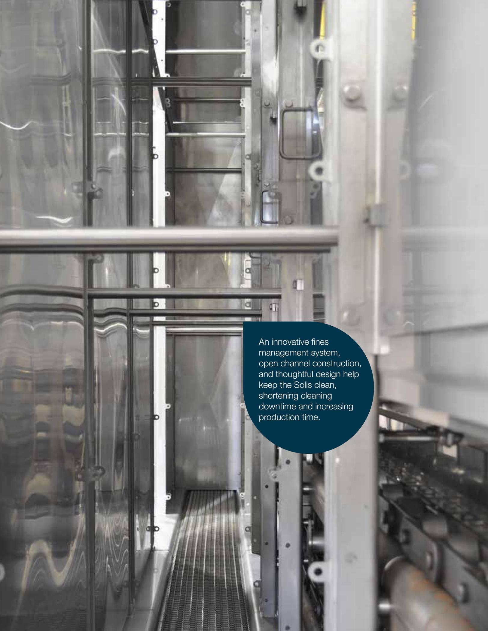
An innovative fines management system, open channel construction, and thoughtful design help keep the Solis clean, shortening cleaning downtime and increasing production time.
